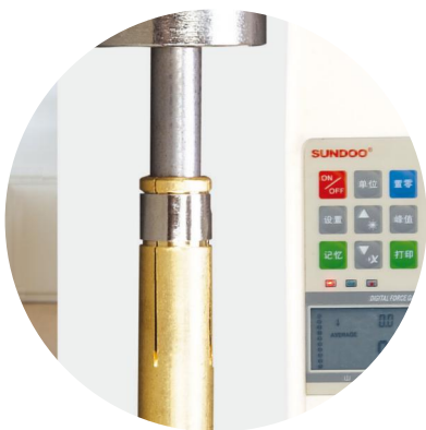
插拔力试验 INSERTION AND EXTRACTION FORCE TEST
