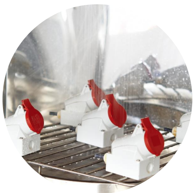
淋雨试验 RAINFALL TEST
